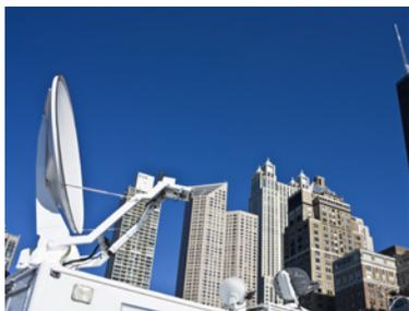
C-band is prized because it is highly reliable and resistant to atmospheric interference. C-band antennas are tuned to receive faint signals arriving from space. As a result, C-band services are susceptible to interference from other telecommunications services transmitting on the ground.
